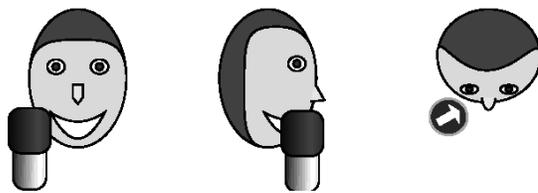
08fig07 An alternate position for a large side-address mic. The arrow indicates the front of the mic, pointing to the mouth.
