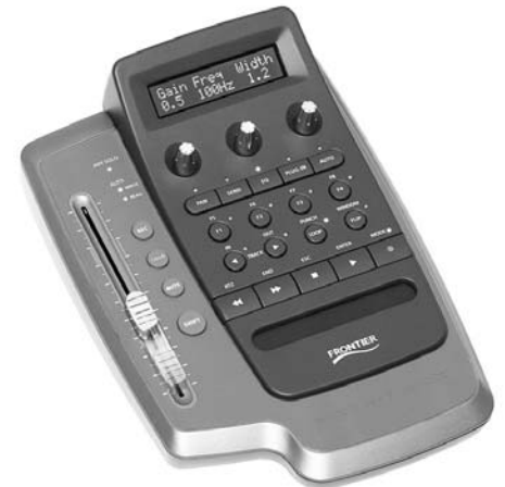
Figure 11.9 A single-fader hardware controller.
