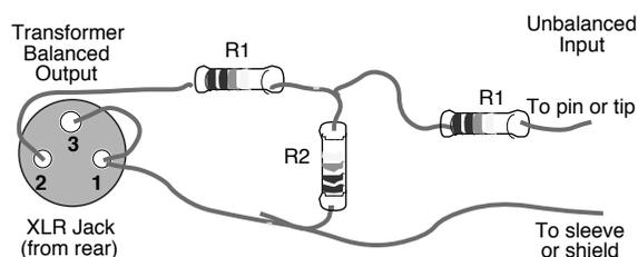
Figure 2: Use this circuit with transformer-balanced outputs
