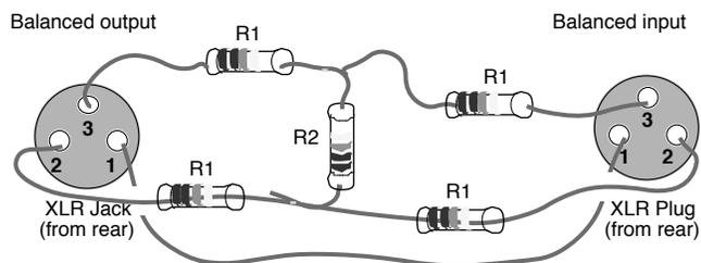
Figure 3: This circuit provides attenuation while keeping the signal balanced
